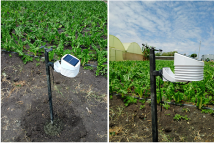
Fig. 4. Deployed prototypes of the mini-weather stations.
